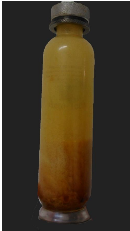
Figure 4.41: Formulation in a glass replica of an aerosol can of PU foam with microcapsules.
